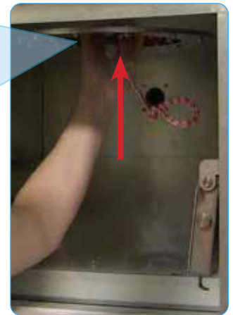
Insert Laser Window Baffle Plug
