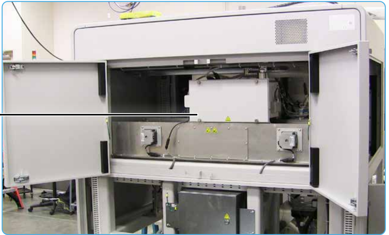
Air Processing Module
