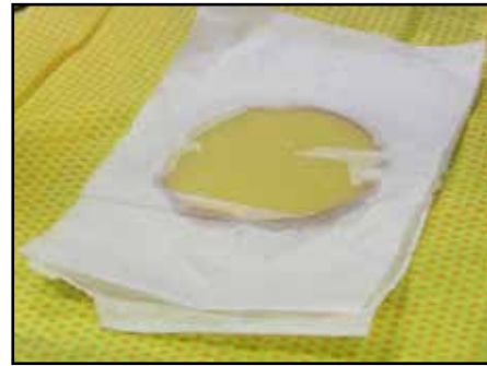
Soak up excess acetone with lens tissue
