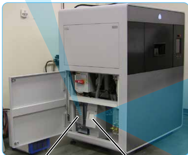
Electrical Enclosure Filters (located on both sides of the enclosure) 2-Stage Hepa Filter (Also located at rear of MQC System)
