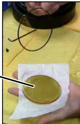
Remove and clean O-Ring
