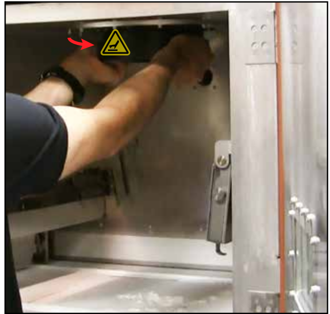
Rotate laser window so label faces forward
