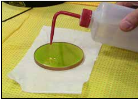
Apply acetone to lens
