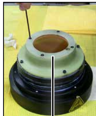
Replace top ring and fasten with 2.5mm allen wrench
